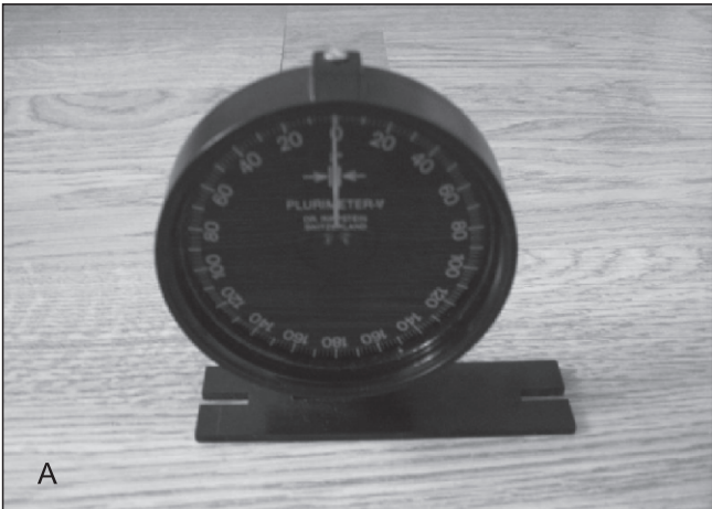
Fig. 1A. Rippstein plurimeter in the “zero” position.
