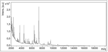
Fig. 1. Sample mass spectrum obtained for E. faecium in the MALDI-Biotyper system (Bruker Daltonics, Germany).
