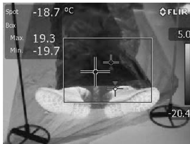
Fig. 2. Thermo-insulation escape routes leading to heat loss – picture taken with thermographic camera; light yellow color states the heat loss areas. Own archive by Tomasz Sanak
