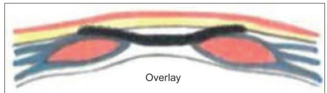
Fig. 7. Overlay mesh location (23)
