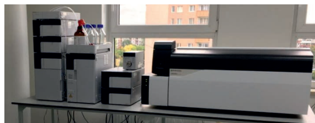
Fig. 2. Example of high performance liquid chromatography coupled with triple quadrupole mass spectrometry
